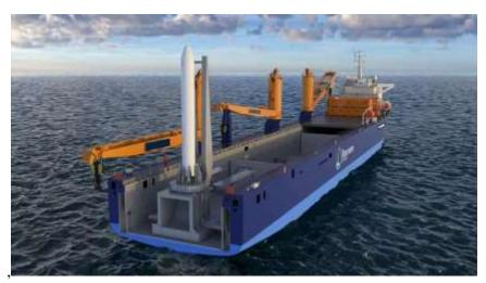
The new German spaceport has little in common with the launch facilities at Cape Canaveral, Florida USA. It will be located on a Roll-on/Roll-off (Ro-Ro) ship. The GOSA RoRo-ship is designed as a floating launch platform with a special ramp and has its home port in Bremerhaven.
